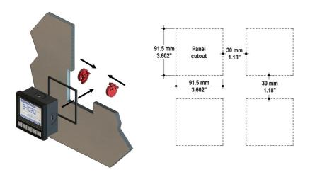
Fix instrument on the panel rotating by hand the fixing snails (M9.SN1).
