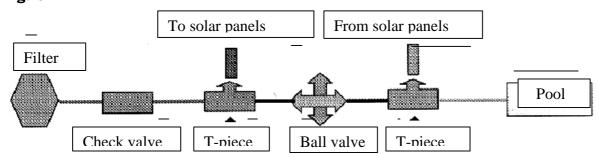
The last thing one has to do is to connect the pipes from the solar panels to the filtration system. These pipes should have at least 55mm and/or 63 mm in diameter. Where possible, our recommendation is to bury the whole system's lines in earth or lead them through interiors. Where the pipes are not buried, make sure they are fastened properly, embedded (best option) into the wall. It is vital as the pipes, when full of water, are very heavy and might suffer damage.
