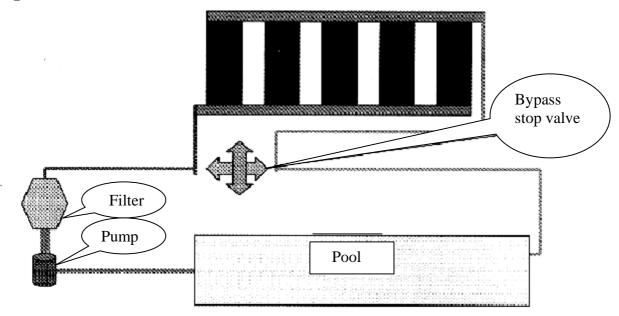
Find a suitable location for connecting the solar system to the water circuit between the filter and pool. See Fig. **"F"**.
