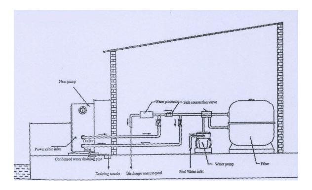
Note: the above piping connection is only an example for demonstration
