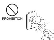
■ If the air-conditioner is not in use for a long time, it is necessary to pull out the power plug. Excessive dust on the power plug may also cause over-heating or a fire.
