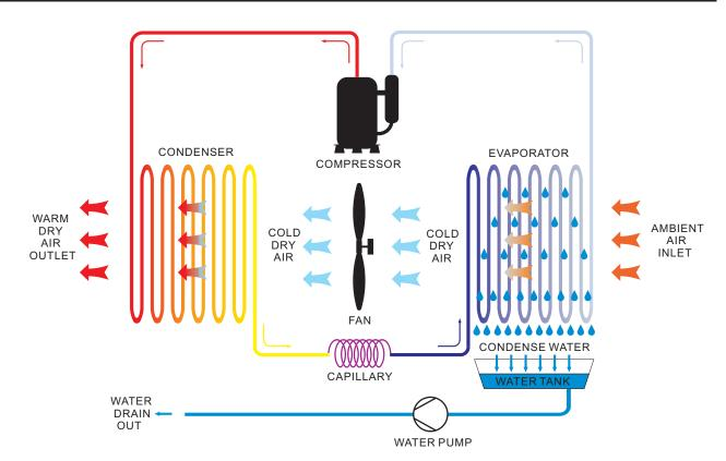
The dehumidifier use the refrigeration circuit to change the damp air warm dry air. When the damp air passes the condenser, the air water will be condensed and the air will become dry.
