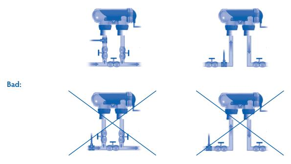
IMPORTANT: The flow sensor must be installed in the right direction (there is an arrow on it showing the flow direction). Make sure it is correctly placed on its connector so that it can stop the Tri salt water chlorinator from producing when filtering is not active (when the red "Flow" indicator is lit there is no flow).).
