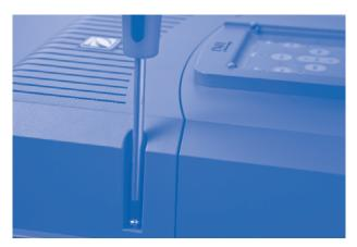
Gently remove the lower module from the TRi unit.
