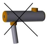
Right – pipe connected in the axis of the connection Wrong – uptight pipe overloads the connection!
