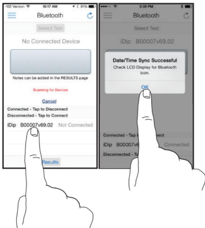
Tap '**SELECT** Test' at the top (e.g. Alkalinity, Total). The iDip and app will both display the test being run.
