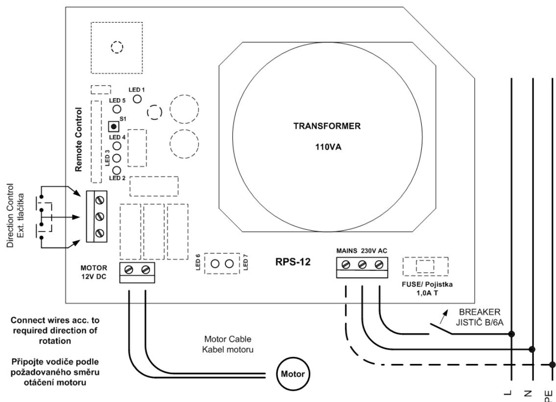
You can control the motor directly by means of a remote transmitting key fob or external dual push button. You can turn off the motor by pressing any button.
