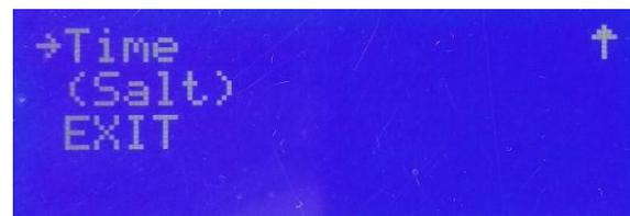
Using the buttons ↓ ↑ you can select a line of the menu, indicated by the arrow (\*). The **OK** button is used to confirm the selection.
